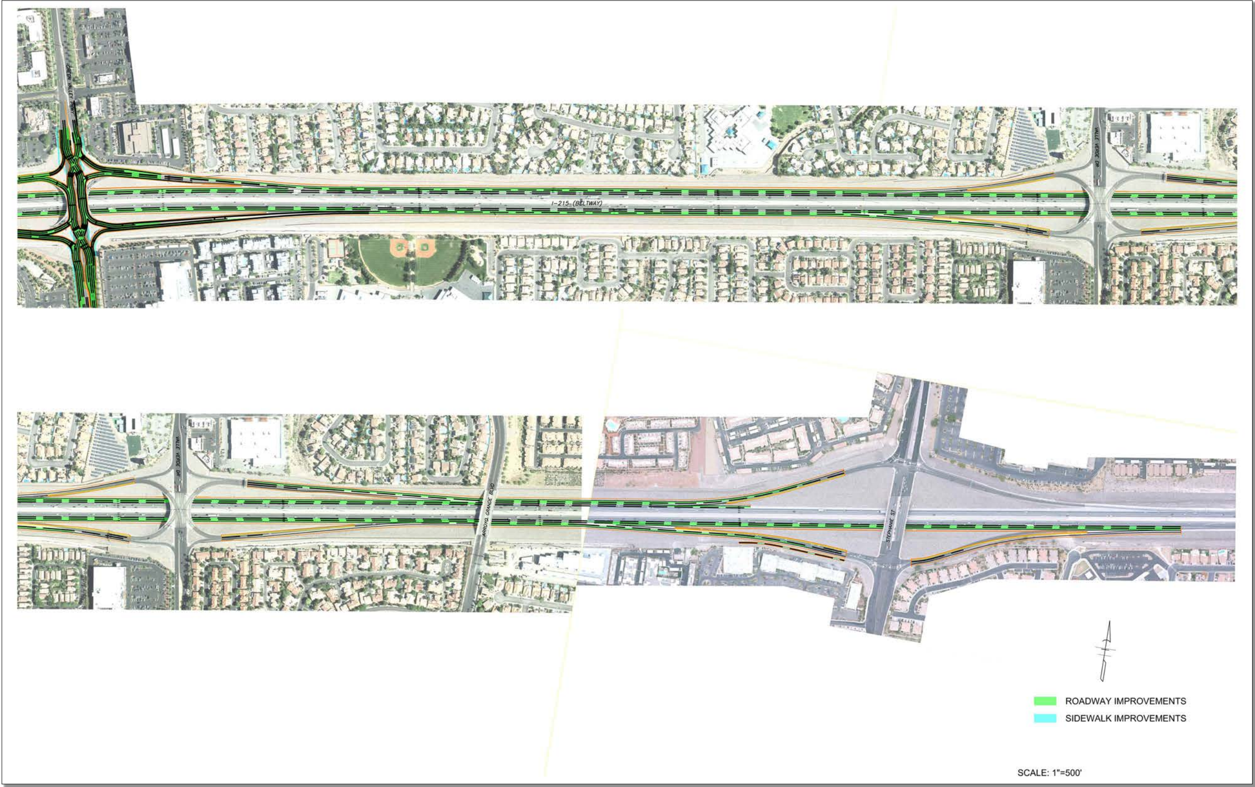
Figure 17: I-215 Improvements between Green Valley Parkway and Stephanie Street – Two Additional Lanes in Each Direction
